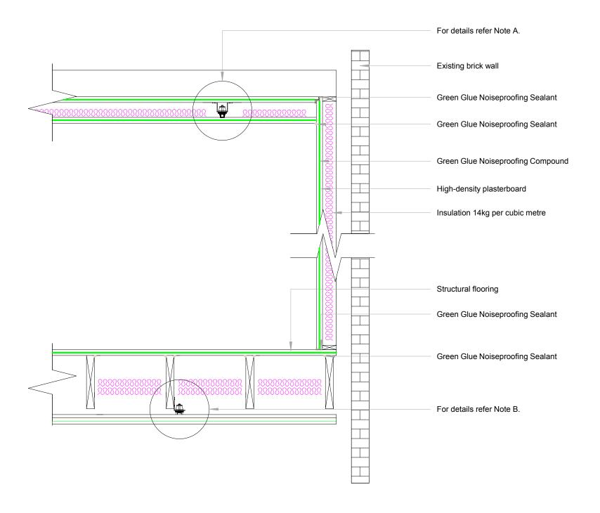
Note A: Soundproofing Construction Guide - Two Layer Ceiling - October 2010
