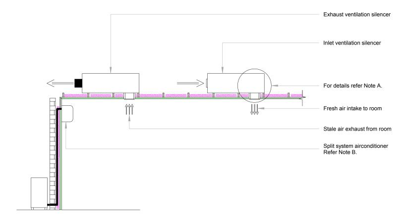
Note A: In terms of soundproofing the ventilation silencer box must be constructed to be as soundproof as the walls and ceiling of the room.
