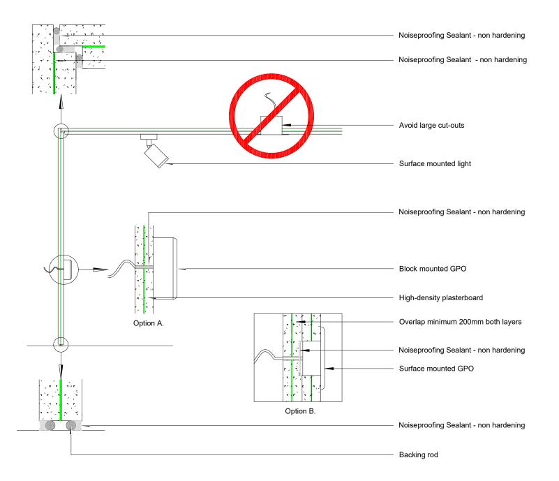
Noise Proofing Sealant to be used on both layers at all joins and penetrations.
