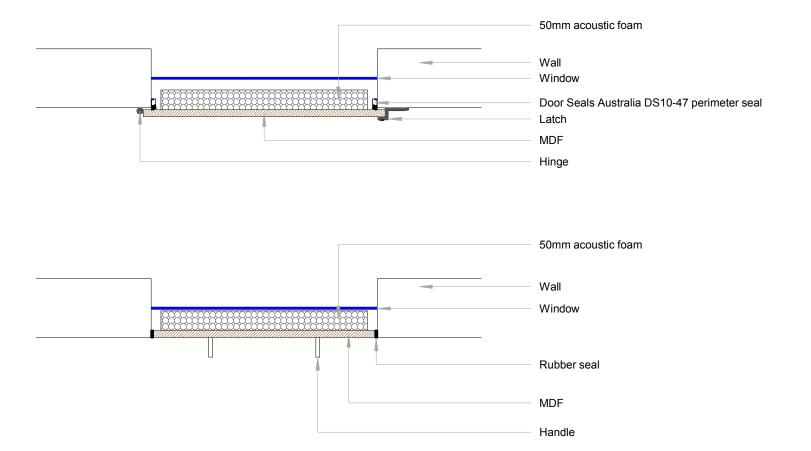
Where recording studio window is not an option, this design works well. It is very important that the seal around all 4 edges of the window be airtight and the cavity be damped with acoustic foam or something similar. This is suitable for windows that need to be opened for light and ventilation but need to be closed at times when it needs to be soundproof.
