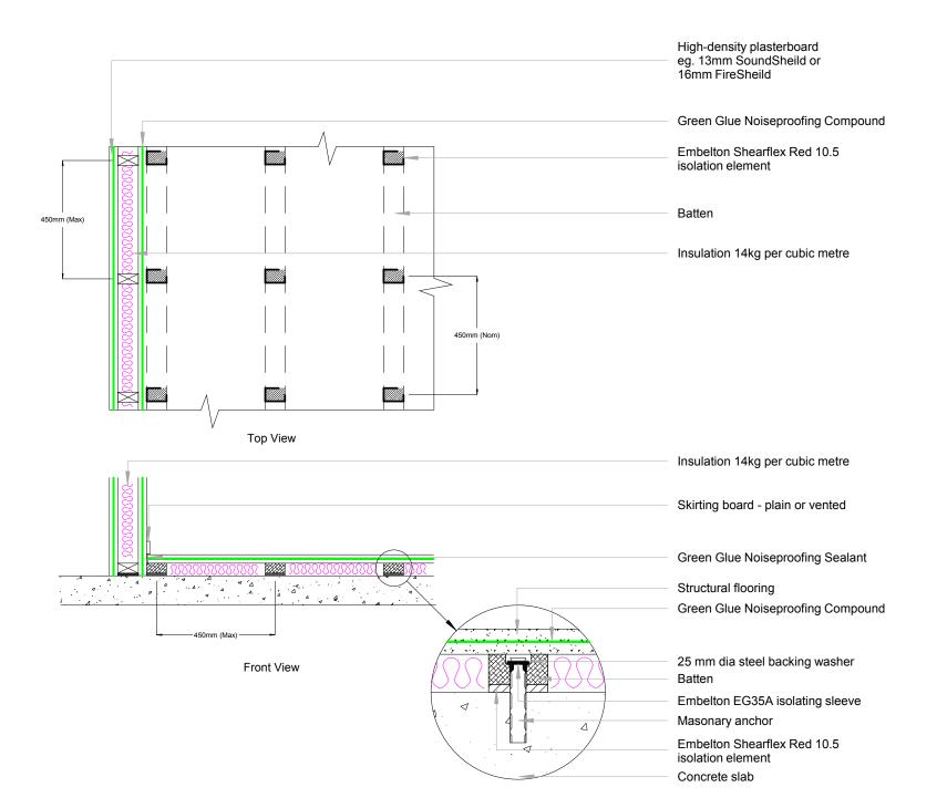
Structural floor should be levelled to +/- 2mm over 1.5m. Use Ardit Z8 or similar.
