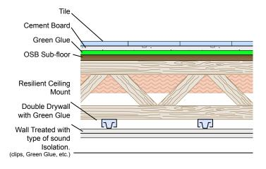
We have lowered costs in the ceiling by removing Green Glue. Even though GG is less costly than clips for a ceiling application, we feel that clips with conventional drywall will outperform GG drywall screwed to the joists for impact noise from tile.
