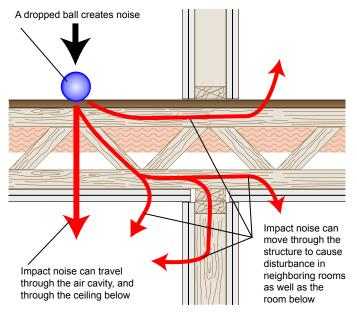
The diagram to the above shows that when we talk about impact noise, we have to talk about structural noise as well as noise passing through the air cavity and ceiling below. Indeed, structure-borne noise is extremely important when discussing impact noise because, by definition, impact noise begins in the structure.
