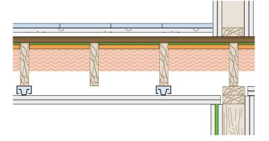
Green Glue sandwiched between the subfloor and strips of HMR or drywall in between the joists.
