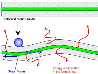
Effect of viscoelastic damping. Viscoelastic damping is unique in that it is effective at reducing noise levels across the entire frequency range with no failure at low frequencies. Damping stands alongside carpet & pad as the only techniques that have no negative impact at any frequency. Its capacity to dissipate energy mitigates flanking noise, helping keep rooms to the side quiet and minimizing structural noise going down.
