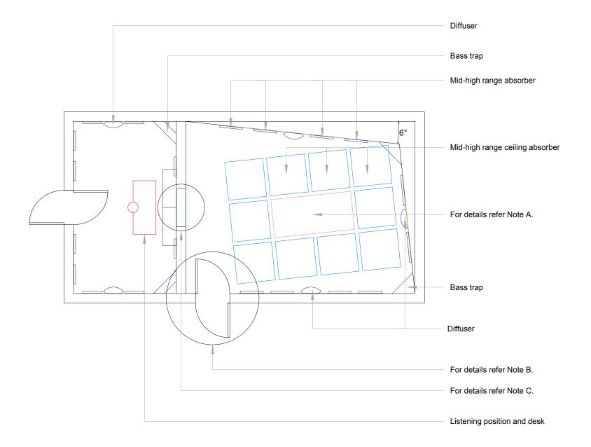
Live Room acoustics need to be adjustable to suit individual artist. All wall modules shown are mounted with Ultrafonic EasyLocate Mounting Rail for this purpose.
